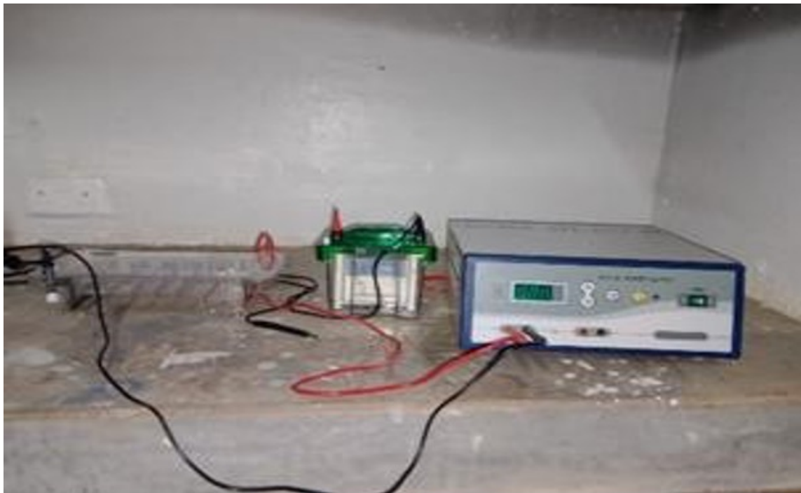
Figure 8. Gel electrophoresis, currently being run by the Biomedical Science students at Laikipia University, Kenya.
