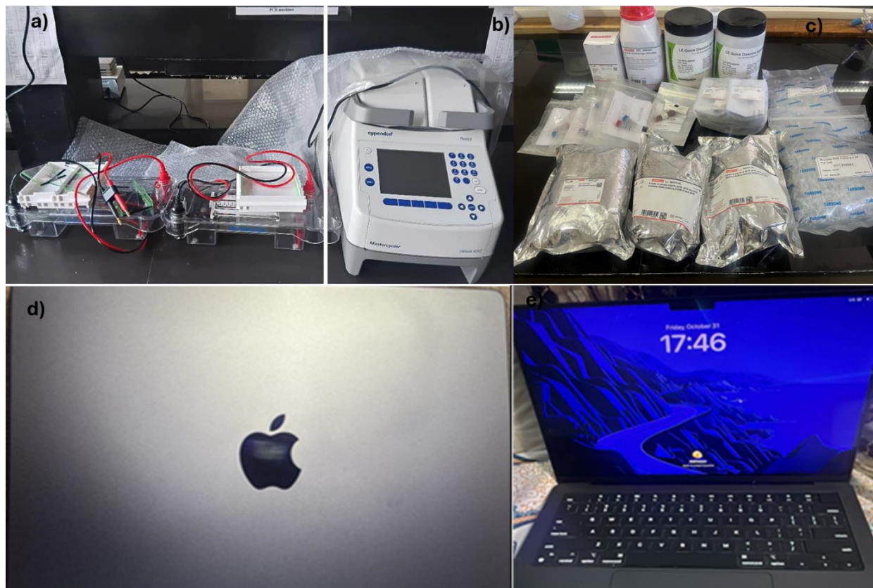
Figure 10. Equipment purchased at Haramaya University, Ethiopia. (a) Mini and Midi gel electrophoresis units, used for the separation of DNA and RNA in a semi-solid agarose gel matrix; (b) Thermal cycler (PCR machine), used to amplify DNA in vitro; (c) Molecular biology reagents; (d) Laptop (MacBook), used by researchers for data analysis generated from laboratory and field experiments.
