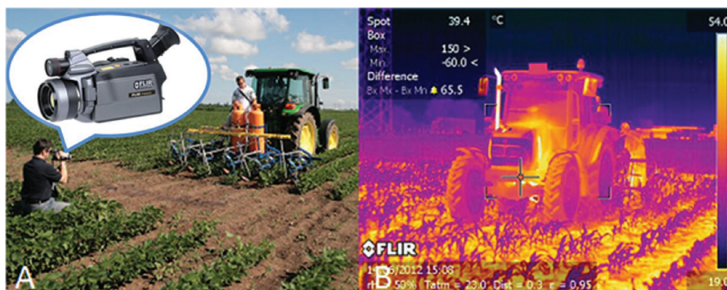
Fig. 9. Temperature measurement with a thermal camera. (A) Thermal imaging in soybean. (B) Thermal image (thermogram) of flame weeding machine. [Photos from Rajković (2018)].
