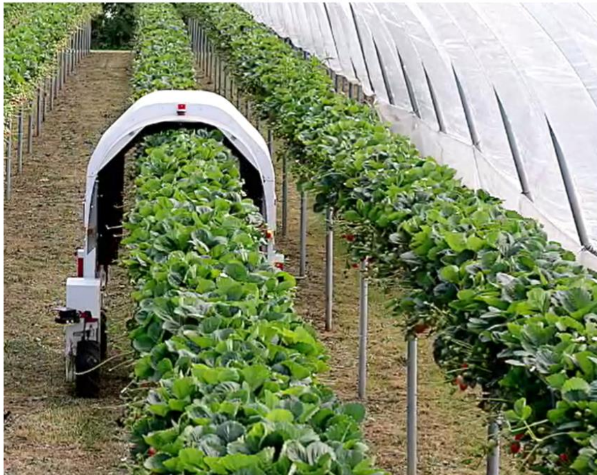
Uv-c application to prevent powdery mildew (Oidium)
