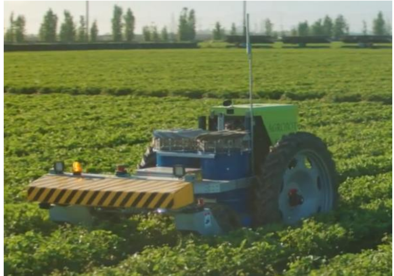
AgroRobot remove bugs through vacuum
